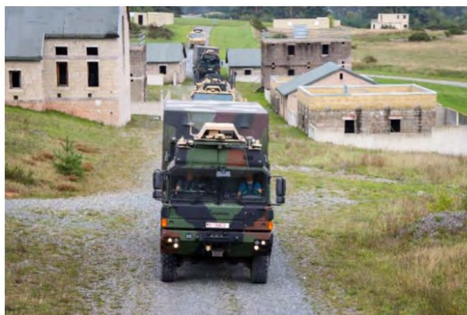
Figure 3 – Rheinmetall-MAN demonstrated leader-follower capabilities using two Rheinmetall-MAN HX2 military trucks fitted with an automation kit Source : The winding path of autonomous vehicles, 2
