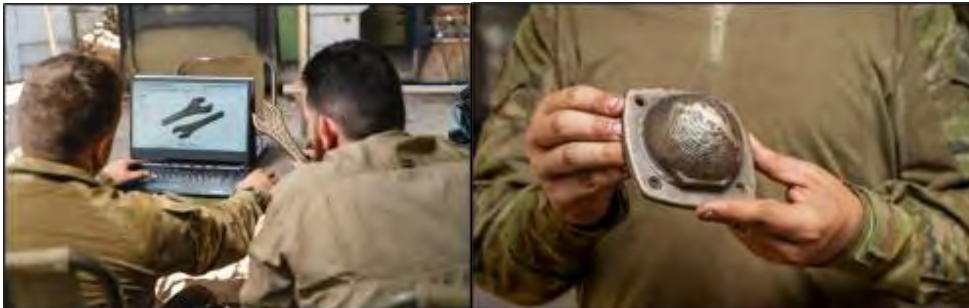
Figure 25. ADF production of 3D metal parts
