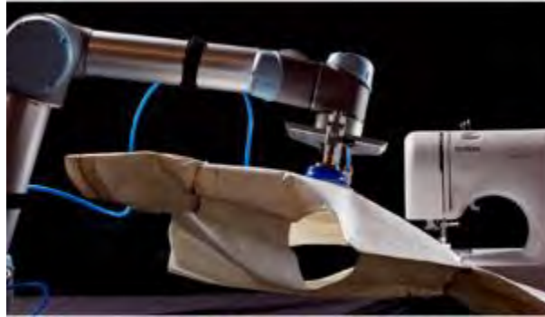
Figure 26 'Sewbo' putting together shirts with little/no human involvement
