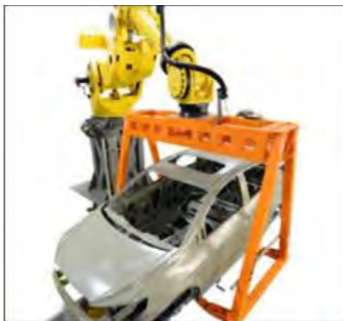
Figure 23. FANUC M-2000iA lifting up to 2300kg
