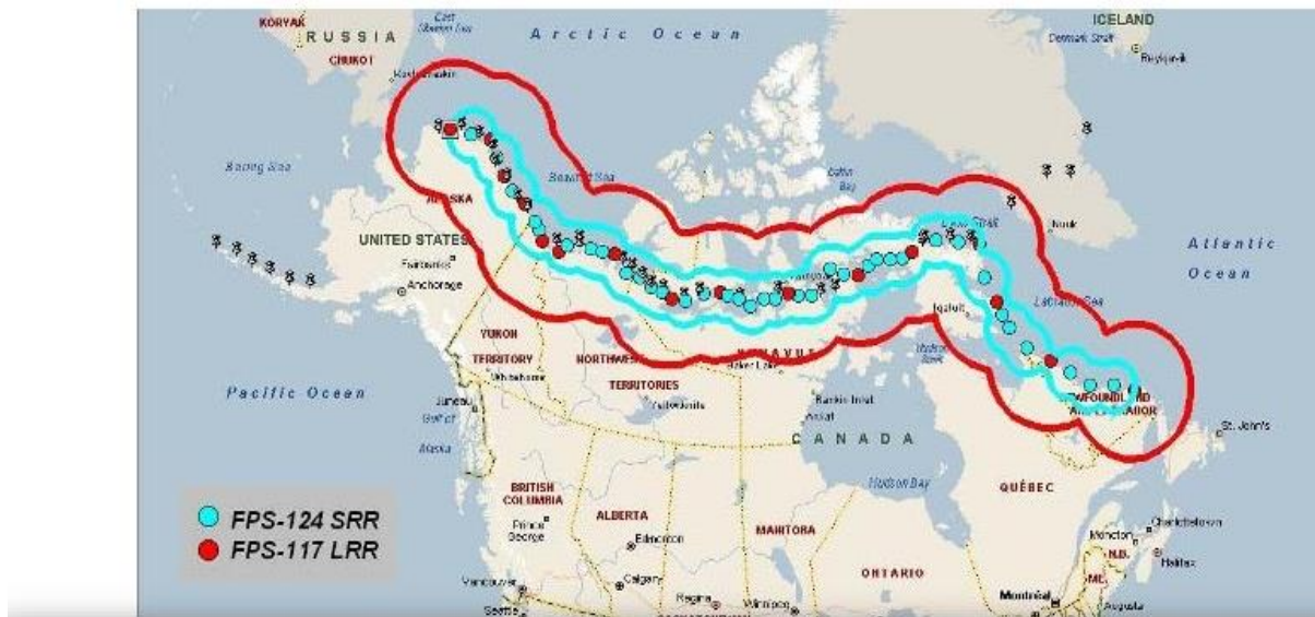
Figure 8. North Warning System coverage map of Canada. The FPS-117 long range radars are shown in red, FPS-124 short range radars in blue. The black "push-pin" icons show former DEW line sites.
