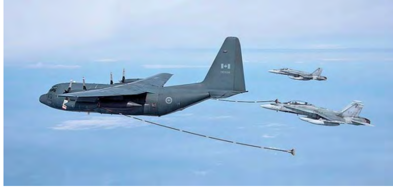
Figure 1 – Probe and Drogue Air-to-Air Refuelling System
