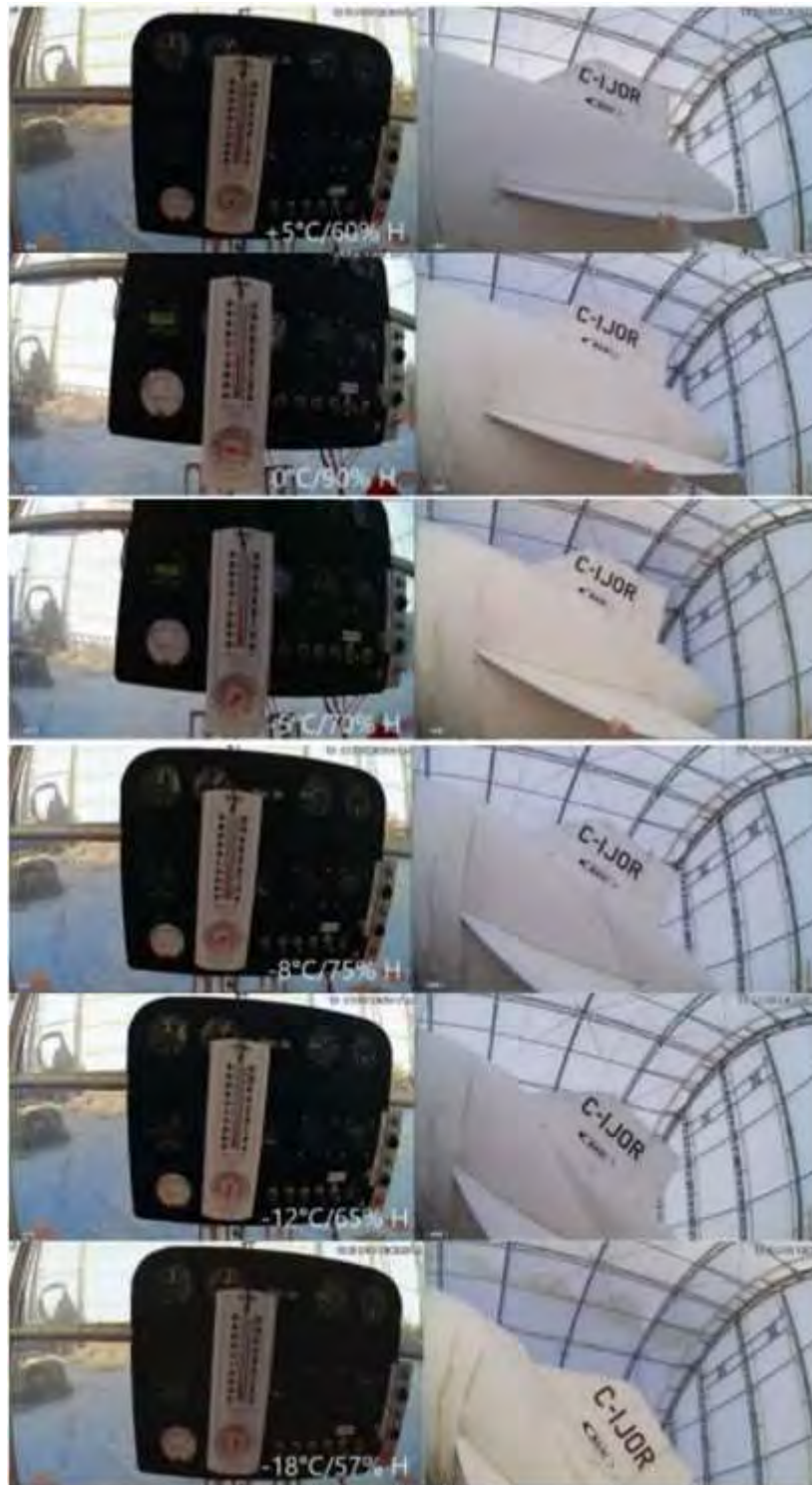
Figure 1.4 – Temperature & Humidity vs. Envelope Deformation Source: Buoyant Aircraft Systems International, Cold Weather Testing
