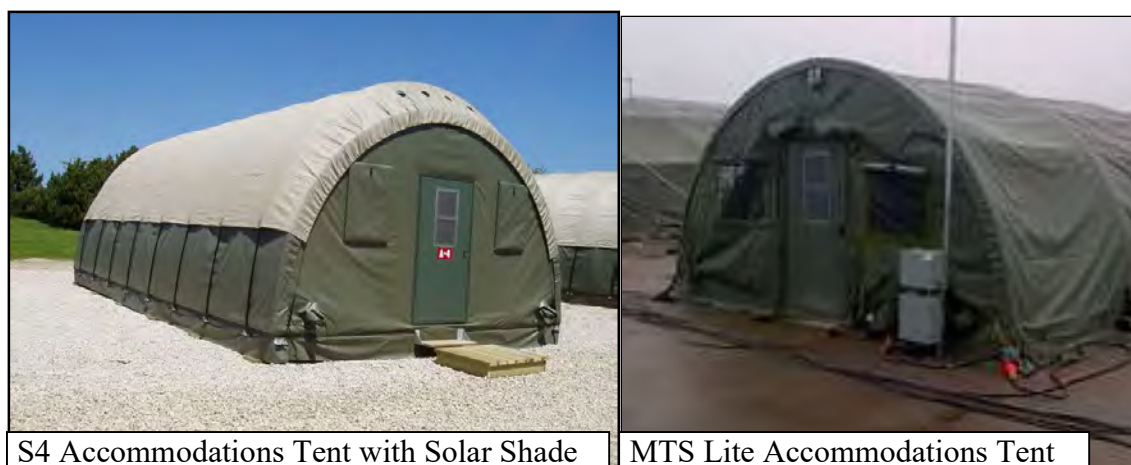
Figure 2.3 – RTC MTS Lite and S4 Weatherhave® Accommodations Tents. Note the S4 has an integral flooring system as well as closer spaced support arches. 33
