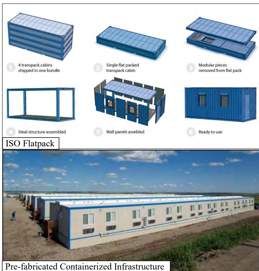
Figure 2.4 – ISO Flatpack 34 and Containerized DFI Solutions. 35
