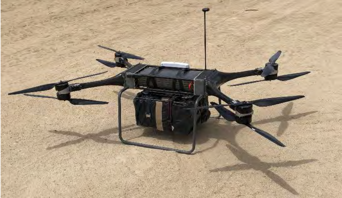
Figure 2: TRV-80 with cargo payload attached
