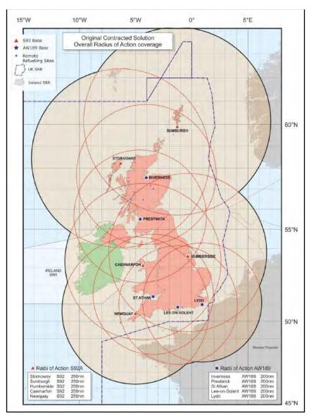
Figure 2 – Map of UK SAR helicopter operating bases with operating radius of 250NM for the Sikorsky S92 and 200NM for the Leonardo AW189.
