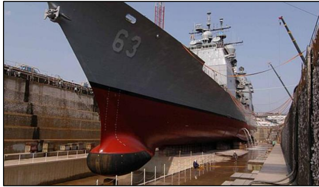
Figure 1 – Example of Hull Mounted Array (HMA) Source: Military & Aerospace Electronics 4
