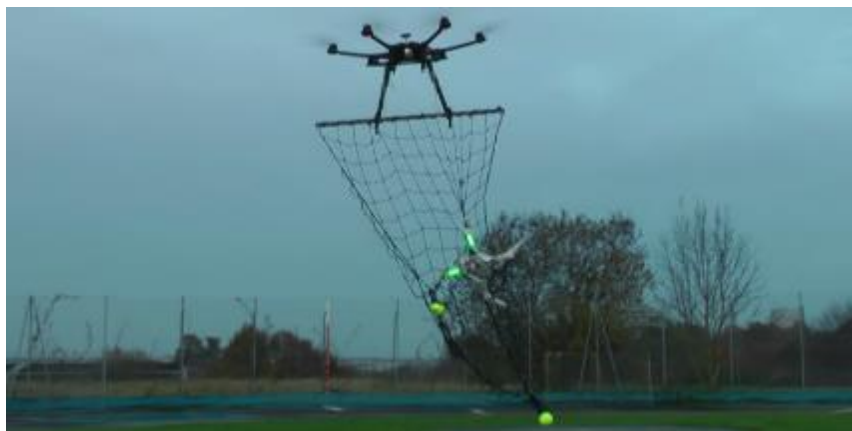
Figure 5.6 - Malou Net Carrying Interceptor sUAS
