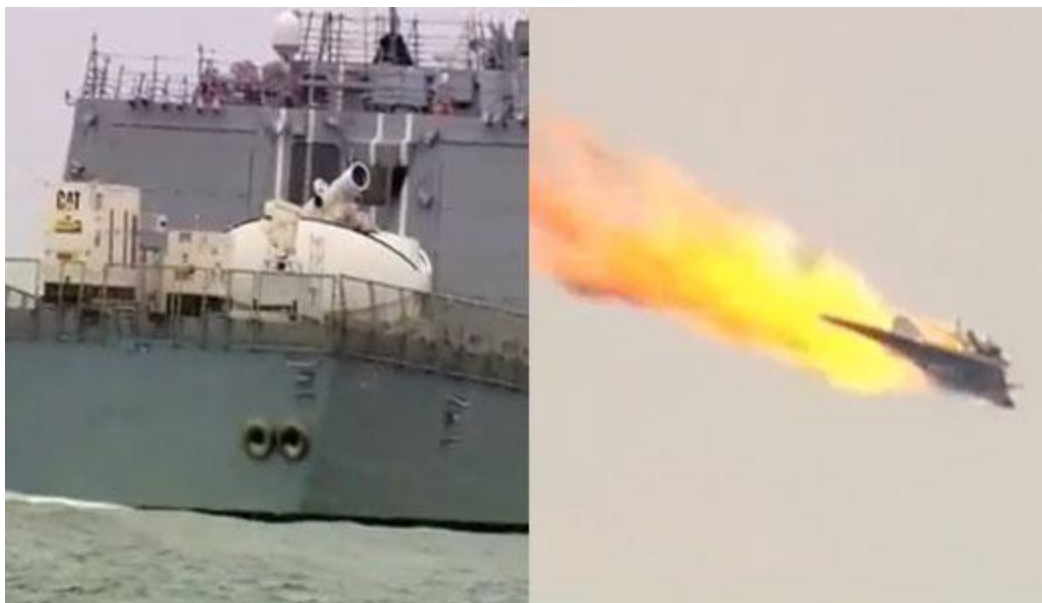
Figure 5.4 - The U.S. Navy's Laser Weapons System (LaWS) and a Successfully Destroyed Target UAS
