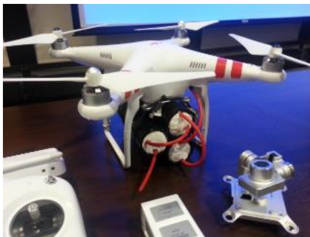
Figure 3.12 - A DJI Phantom 2 rigged with a mock explosive payload
