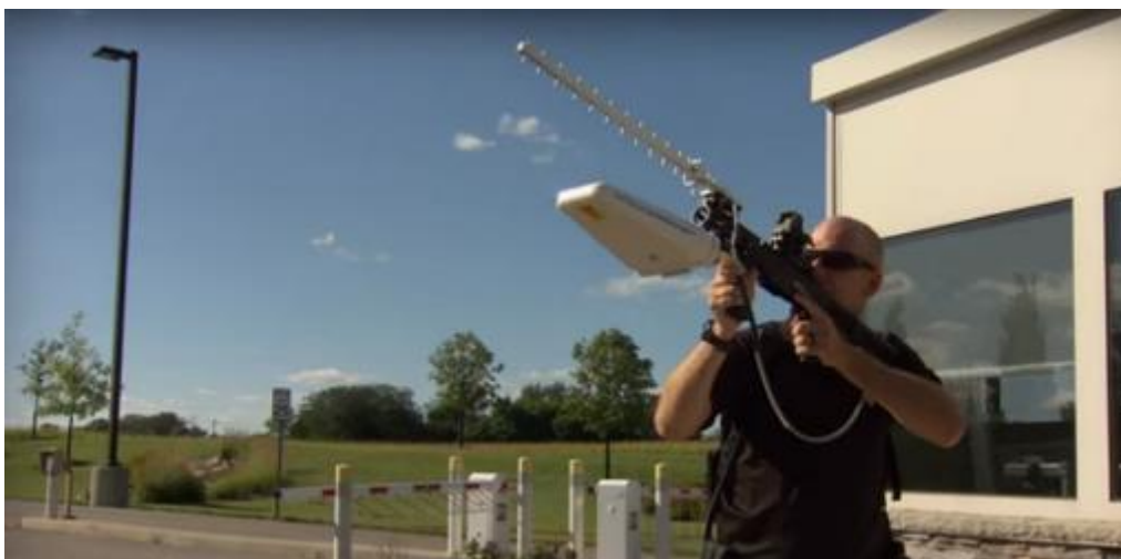
Figure 5.7 - Battelle's DroneDefender Jamming System
