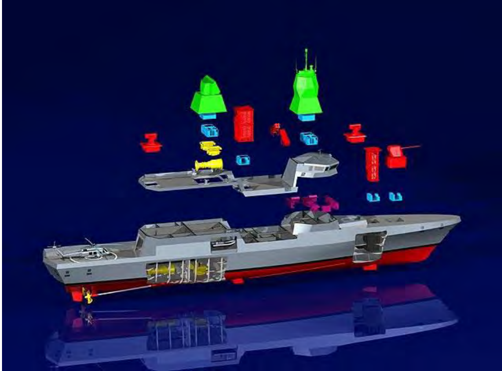
Figure 25 - Bloom + Voss MEKO Modular Design
