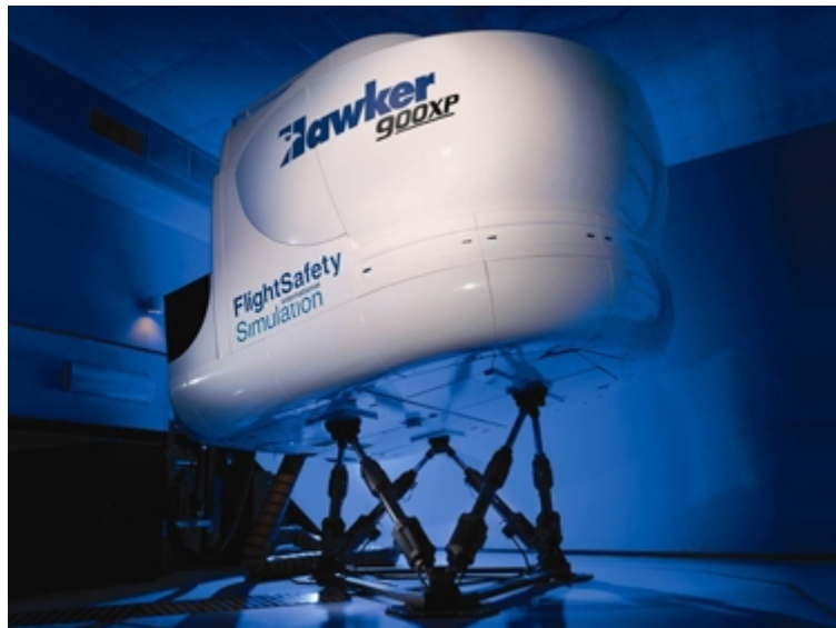
Figure 2.6: Modern 6 Degrees-of-Freedom Motion Simulator Source: http://www.amtonline.com/article/article.jsp?id=7781&siteSection=1
