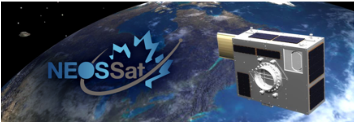
Figure 5.1: Image of the 65 kg Near Earth Orbit Surveillance Satellite (NEOSSat) designed by the CSA and DRDC for dual missions. Under the auspices of CSA’s Near Earth Space Surveillance program out of the University of Calgary it will carry out NEO Detection and Tracking of ATEN and Apollo orbiting PHA. It will also define the resident debris objects occupying the High Earth Orbit (HEO, from 10,000 to 37,000km above the Earth). (Figure Credit: Canadian Space Agency)
