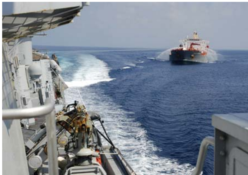
Figure 4 – Tanker ship with fire hoses rigged to repel pirates 89
