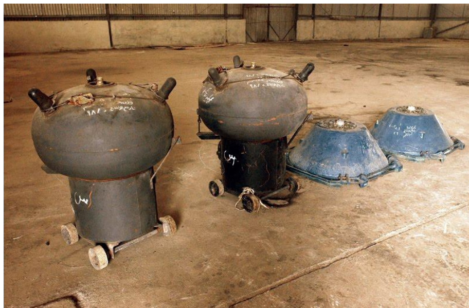
Figure 2 - Iraqi Sea Mines. Iraqi LUGM-145 Moored Contact (left) and Manta Ground Influence (right) sea mines.
