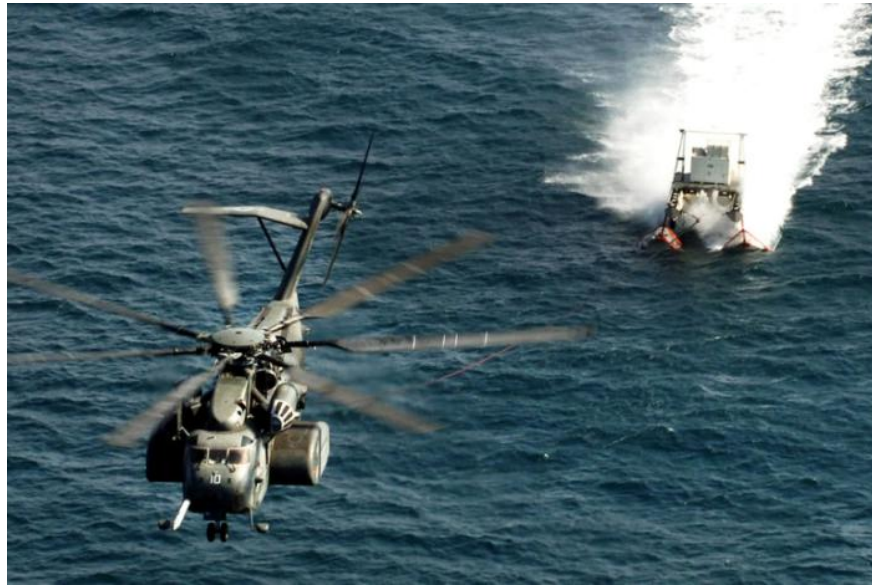
Figure 11 – Air NMCM. USN MH-53 Sea Stallion NMCM Helicopter, towing a MK105 Magnetic/Acoustic Influence Sled.
