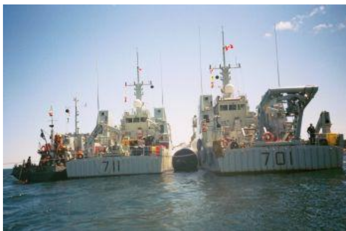
Figure 26 – ROV Operations. Two Kingston Class Ships positioned over a disabled submarine during a SUBSUNK Exercise. HMCS Glace Bay (right) has the DSIS deployed.
