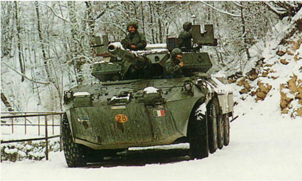
Fig 3.2: The Italian Centauro 105 mm prototype (Light Armoured Tank with 105 mm cannon). Photo taken from Centauro web page (photographer unknown).
