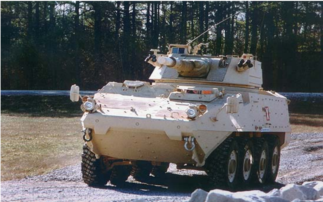
Fig 3.4: The Piranha III Prototype (Light Armoured Tank with 120 mm smooth bore cannon). Photo taken from Piranha's web page (photographer unknown).
