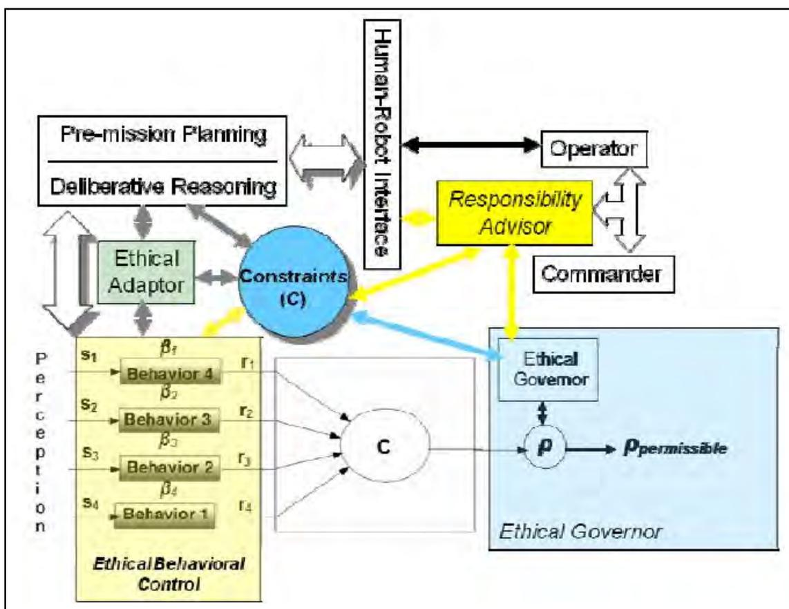
**Figure 5.0: Major Components of an Ethical Autonomous Robot Architecture.**
